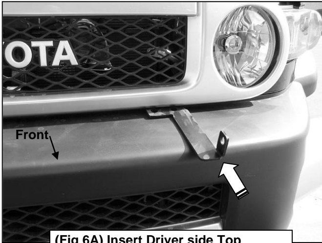
(Fig 6A) Insert Driver side Top Bracket through gap above bumper
