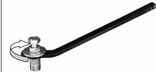
(Fig 5B) Assemble 6mm Insert Tool
