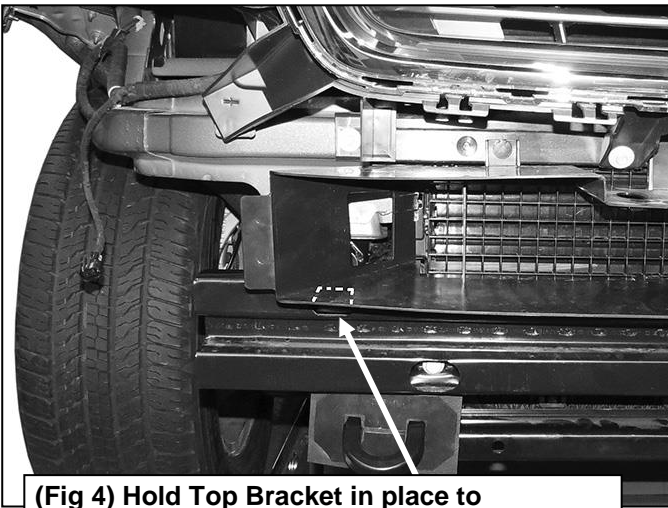
(Fig 4) Hold Top Bracket in place to determine area to cut from air deflector
