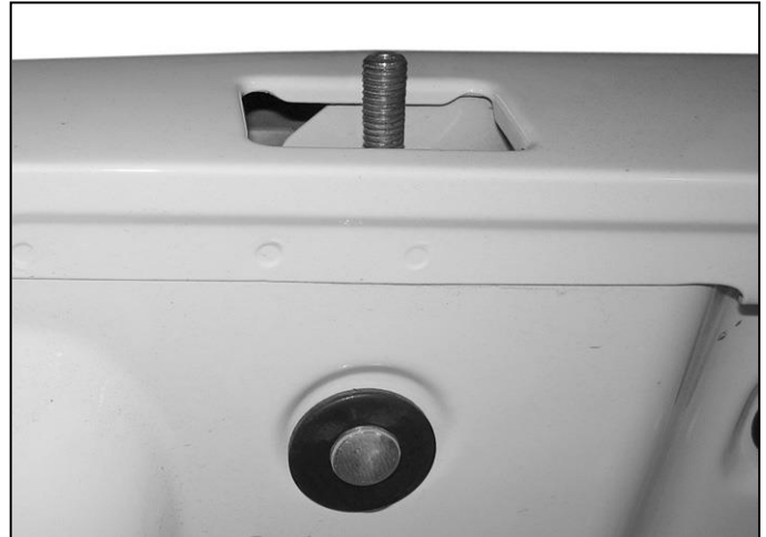
(Fig 4) Use the "J" Bolt to secure the front mounting holes on the Bracket to the stake pocket if possible. Do not drill any mounting holes until after all mounting locations are checked for clearance
