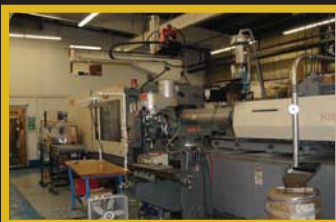
★ Molding in polycarbonate, ABS, Glass Filled Nylon and Over Molding in Polyurethane, Press capability from 80 - 700 tons ★ Color Blending capability at the presses, chromaticity validation for color
