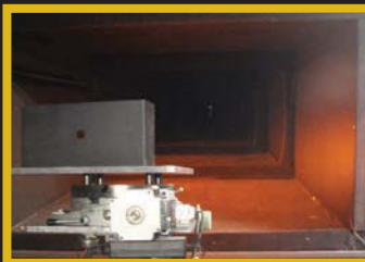
★ Light Tunnel: Photometric Validations to SAE standard for LED, Fluorescent, Strobe, Halogen and Incandescent ★ Meets the requirements of Automotive, Emergency Equipment, Rail, Industrial Fire Alarms, Certified by AMECA
