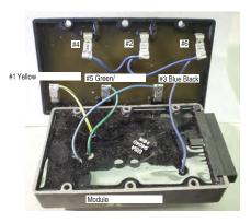
Attach the module wires as shown to the coil. Be careful to not flex the terminals more than necessary to avoid breaking them. Once all terminals are connected, fold them over so they lay flat against the bottom of the coil. Install the coil to the module.
