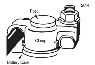
A fully seated battery clamp makes contact with the battery case.
