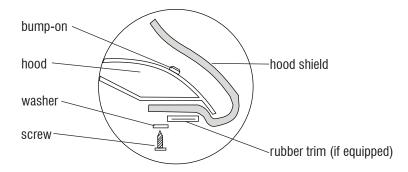
**IMPORTANT:** Before driving, ensure the hood shield is properly secured to vehicle. Clean with a **SOFT** cloth and soap and water ONLY! Using abrasive cleaners, chemicals, or solvents will **VOID** the warranty on this product.
