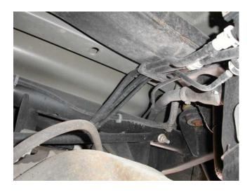
5. After rerouting of the EVAC tubes, you will have the necessary clearance for the installed overaxle true dual pipes to fit through this area of the vehicle. Below is a picture of the rerouted EVAC tubes.
