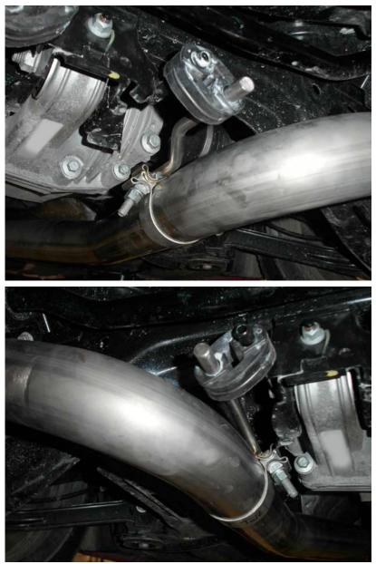
25. Take factory mufflers and cut muffler inlet pipes removing just the flared pieces and deburr. See picture of cutoff flared piece below.
