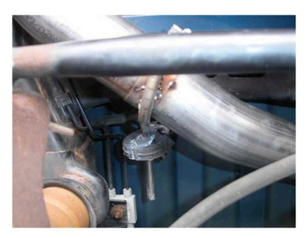
15. Install the two remaining 3" hanger clamps- one on each tailpipe.
