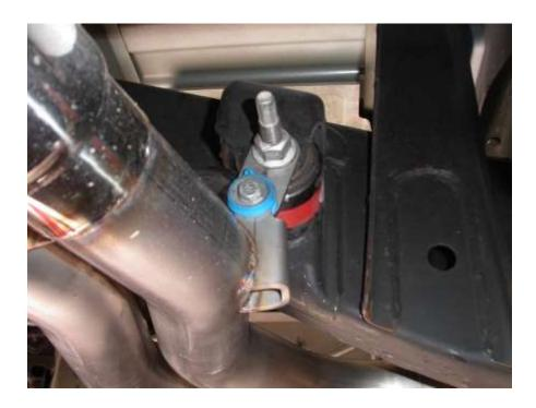
9. Install tail pipes and tips using (2) 3" clamps and grommet with 3/8" bolt, washers and nut.
