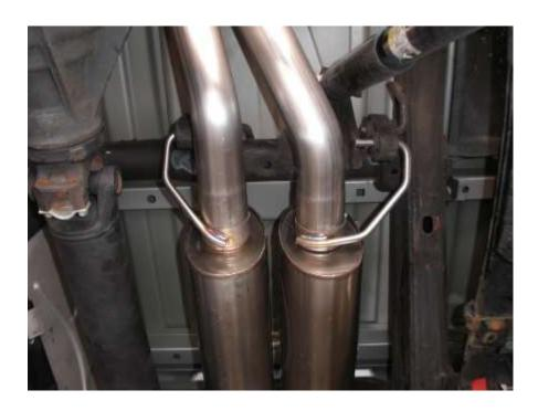
9. Install Right and Left tail hangers to factory bolts in trailer hitch using farthest ones forward 14mm, (see picture).
