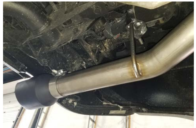
Detail 12: Rear tail section and tip installed.
