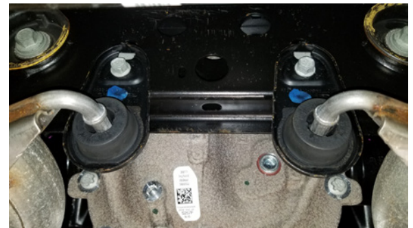
Detail 5: Rear subframe hangers
