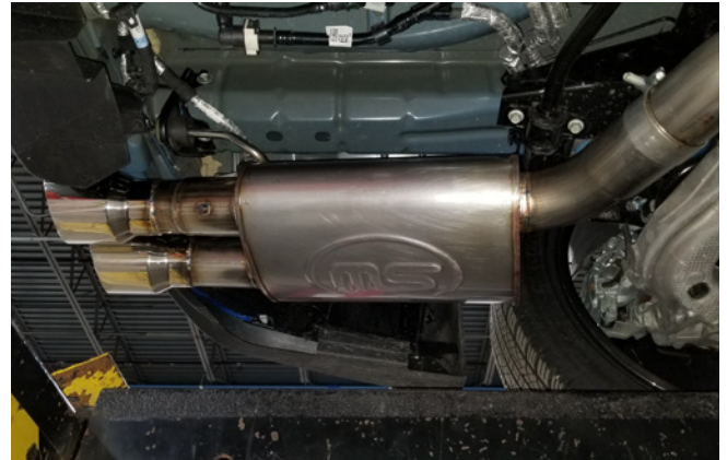
Detail 12a: Left muffler assembly installed
