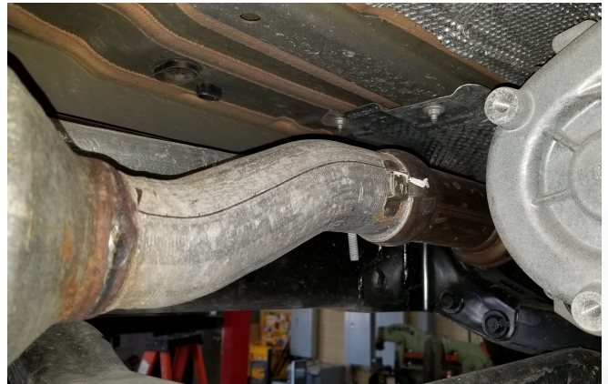
Detail 7: OEM catback connection
