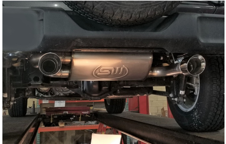
Detail 15a: Muffler and tips installed
