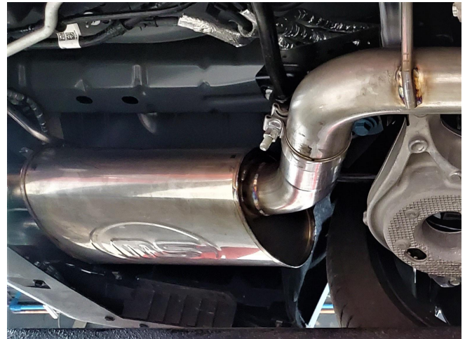
Detail 12a: Left muffler assembly installed
