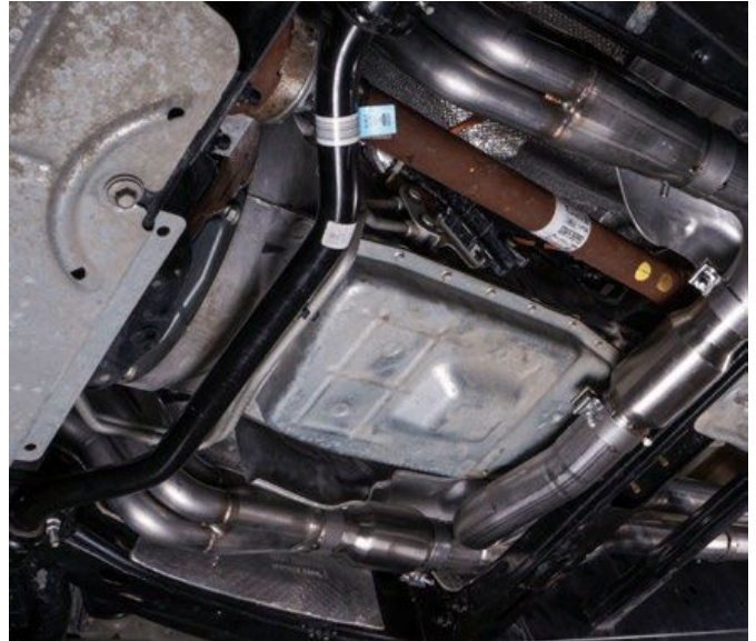
Installed headers close-up
