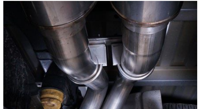
Detail 9: Front tailpipe hanger
