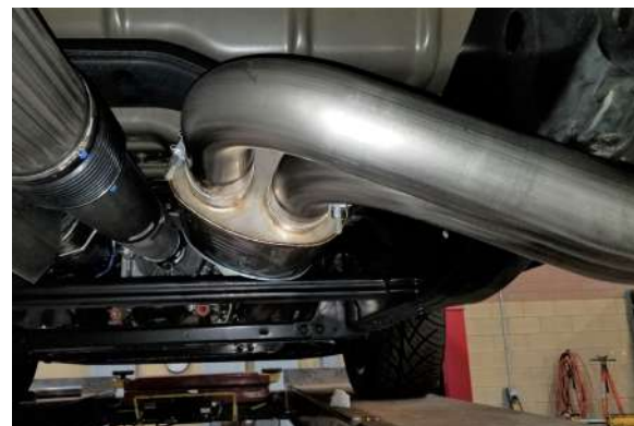
Detail 10a: Tailpipes installed to muffler.
