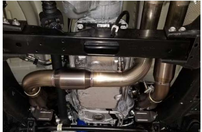
Detail 16: Headers and leads installed
