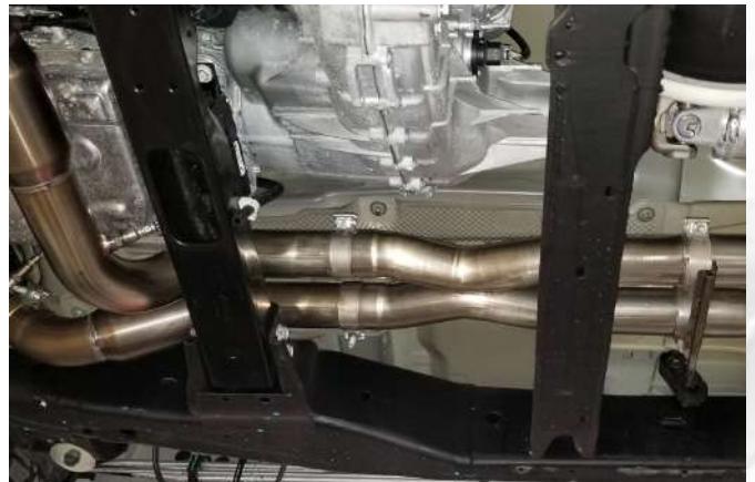
Detail 17: Catback connection (shown with SW catback)
