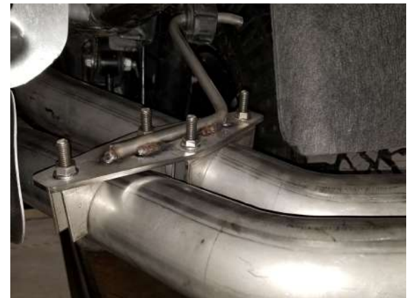
Detail 16: Tail hanger viewed from rear of vehicle.
