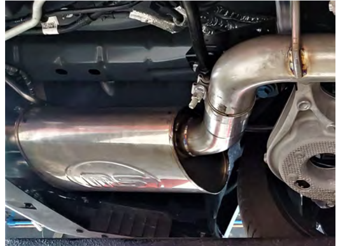
Detail 12a: Left muffler assembly installed
