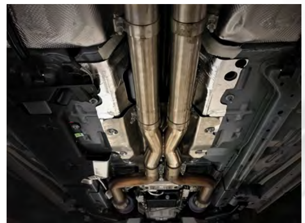
Detail 9: X-pipe and mid pipes installed (factory connect shown)
