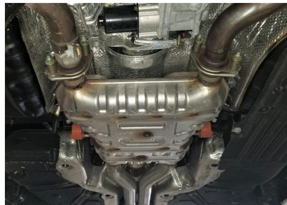
Detail 5: (4) nuts at catback connection
