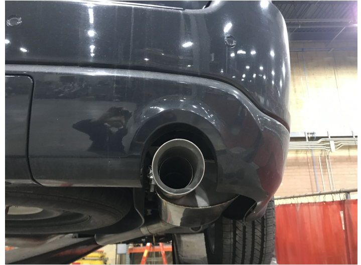
Detail 12: Right muffler assembly with tip installed
