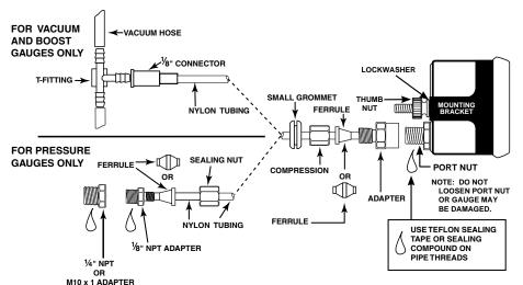
NOTE: DO NOT OVER TIGHTEN ADAPTER FITTING OR GAUGE MAY BE DAMAGED.
