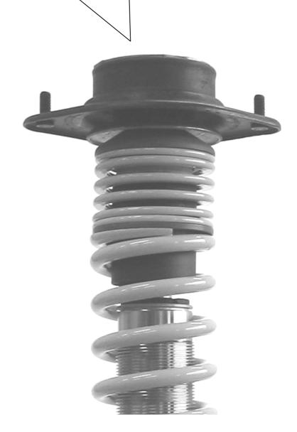
After you have completed installation of the suspension, check the clearance of the tyres to the front suspension strut. The minimum clearance at the narrowest point is 5 mm and must, where necessary, be provided using commercially available, Technical Inspectorate (German TUEV) approved spacers.
