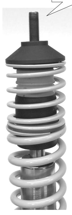
Put on the original supporting bearing, as shown on the picture, and srew it with the original hexagon nut. The original underlay disk, which is put between original spring perch and piston rod, is not necessary. To install the coilover strut in the vehicle use the supplied stop nut. Tightening torque for the piston rod is 50 Nm (37 ft-lb). Please install the strut unit to manufacturers recommended settings regarding tightening torque and fixing specifications.
