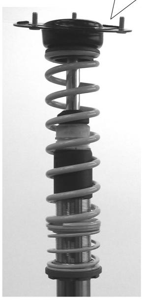
After you have completed installation of the suspension, check the clearance of the tyres to the rear suspension strut. The minimum clearance at the narrowest point is 5 mm and must, where necessary, be provided using commercially available, Technical Inspectorate (German TUEV) approved spacers.
