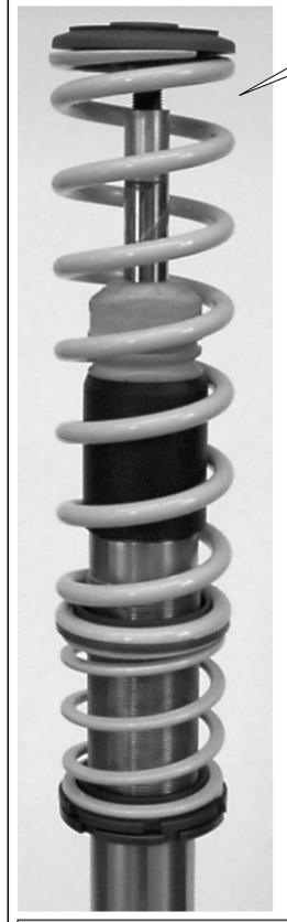
Put the original top mount on the spring perch and fix it with the supplied nut. Tightening torque to 60Nm. Please take the information for the installation of the coilover strut into the vehicle from the documents of the vehicle manufacturer. Remove the original spring support.
