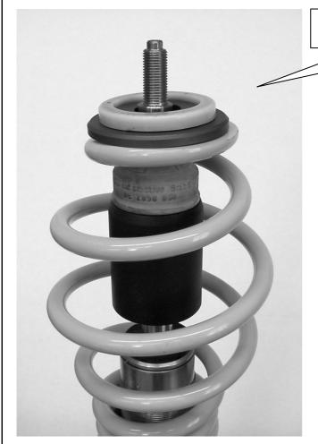
Supplied complete front coilover strut with supplied original axial bearing.
