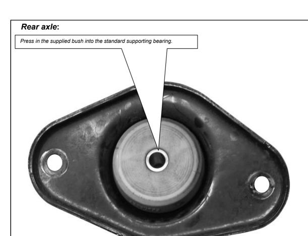
The orginal HA supporting bearing has a mark for the righte side = R and the left side = L. Please installation the Supporting bearing on the corect side.
