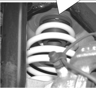
Unless there is no spring (Elastomer) supplied by the factory spring (Elastomer) has to be used. The factory spring (Elastomer) has to be in a good condition, otherwise it has to be replaced. Therefore only use spare parts for BMW E46 M-technic. Tightening torque for piston rod nut is 25 Nm (18 ft-lb). The rear axle shock absorber has to be installed according to the car manufacturers installation instructions.
