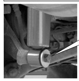
Use the supplied washer at the lower damper fixing point. Install the washer facing the center of the vehicle (as shown on the picture). The rear axle shock absorber hast to be installed according to the car manufacturers installation instruction.
