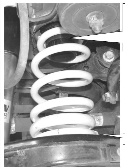
Mount the rear axle adjustment between spring and chassis, the original spring support is no longer used. You have to remove the rear axle adjustment to correct (screw up the threaded ring) the car height. Attention: Before the installation of the height adjustment perch the touching surface area have to be cleaned.
