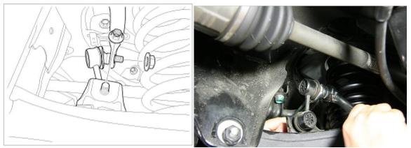
**2b.** Remove the original equipment bushing brackets as well using a **14mm** socket. Note the position of the anti-sway bar in the vehicle to ease in the installation of your new Suspension Techniques Adjustable Anti-Sway Bar. Carefully remove the original equipment anti-sway bar from the vehicle by sliding the end-link out of one side of the bar and pulling the bar out.
