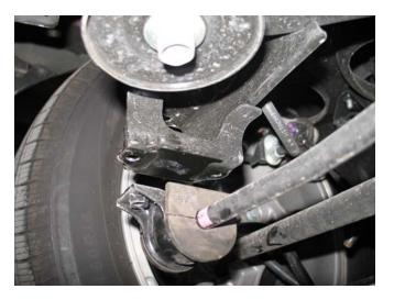
**8.** To remove the original equipment swaybar you must first remove the driver's side, then turn the swaybar towards the front of the vehicle and rotate the swaybar to remove it from the passenger side.
