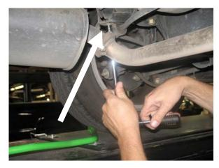
**8.** Position your new ST Anti-Sway Bar on the vehicle, (photo 4), install the O.E. end link, but do not totally tighten, to one of the holes on the end of the Anti-Sway Bar. Use the same hole on each side.
