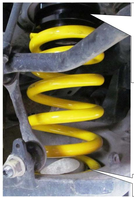
Mount the rear axle adjustment between spring and chassis, the original spring support is no longer used. You have to remove the rear axle adjustment to correct (screw up the threaded ring) the car height. Attention: Before the installation of the height adjustment perch the touching sur-face area have to be cleaned.
