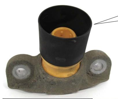
Press the supplied stop element with dust protection tube into the standard support bearing.
