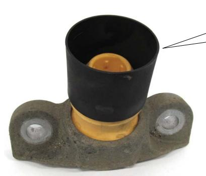
Install the original supporting bearing and fit with the standard nut. Please install the damper unit to manufacturers recommend-
