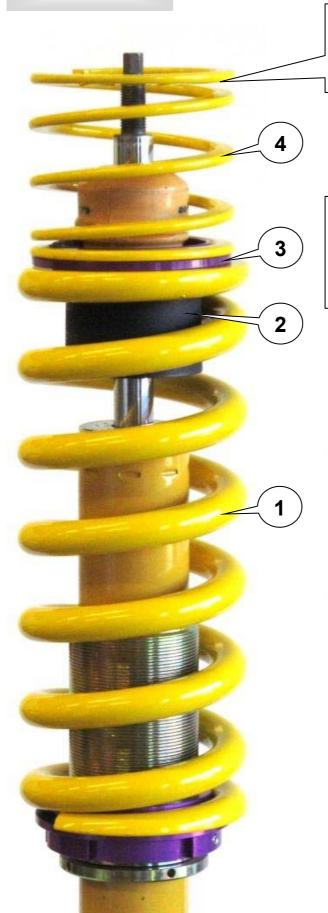
Insert the following supplied parts in the same succession: spring  ${\bf 1}$ , bumpstop with dust cover  ${\bf 2}$ , Intermediate ring  ${\bf 3}$  and Helper spring  ${\bf 4}$ .
