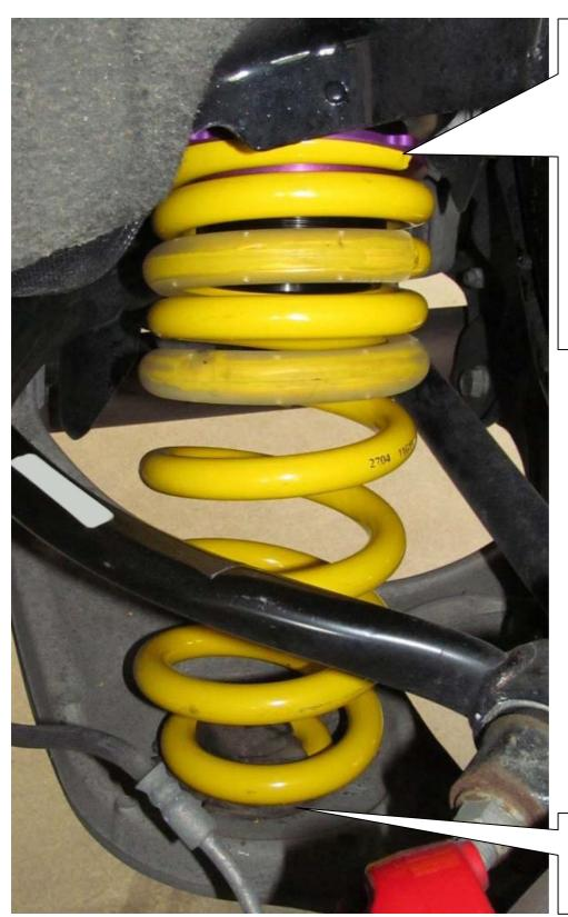
Mount the rear axle adjustment between spring and chassis, the original spring support is no longer used. You have to remove the rear axle adjustment to correct (screw up the threaded ring) the car height.
