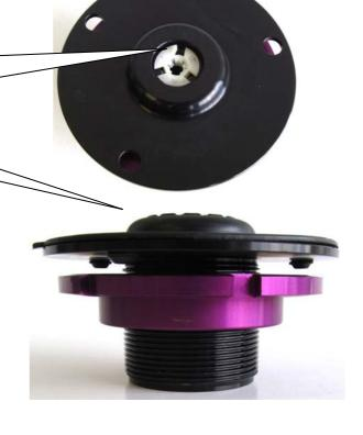
Use the original spring support at the bottom end of the spring.
