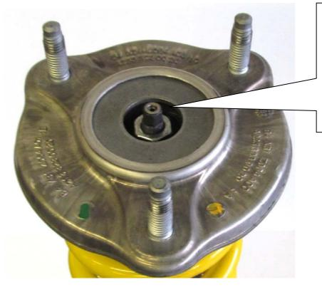
Install the original supporting bearing and fix it with the standard nut. Please install the strut unit to manufacturers recommended settings regarding tightening torque and fixing specifications.
