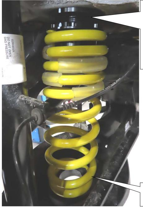
Mount the rear axle adjustment between spring and chassis, the original spring support is no longer used. You have to remove the rear axle adjustment to correct (screw up the threaded ring) the car height. Attention: Before the installation of the height adjustment perch the touching surface area have to be cleaned.
