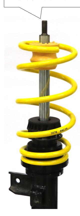
Install the factory top mount with dust cover and secure it with the OEM nut. The strut unit has to be installed according to manufac-turers instructions settings regarding tightening torque and fixing specifications.
