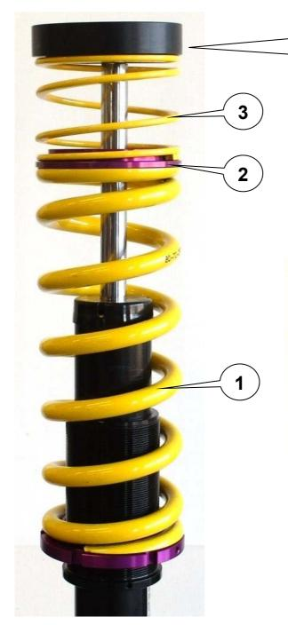
Insert the following supplied parts in the same succession: spring  ${\bf 1}$ , Intermediate ring  ${\bf 2}$  and Helper spring  ${\bf 3}$ .
