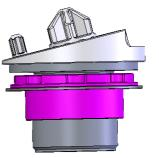
The height adjustment with adapter has to be inserted at the top and the original upper spring support has to be removed. Please read the height adjustment for adjusting the car height.
