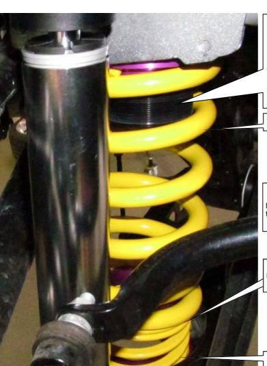
Mount the rear axle adjustment between spring and chassis. Remove the original spring supporting disc. You have to remove the rear axle adjustment to correct (screw up the threaded ring) the car height.
