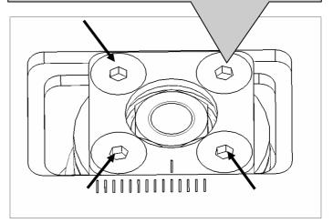
Note camber adjustment: Adjust the uniball supporting bearing to the middle adjustment (position like original supporting bearing). If the camber needs to be adjusted during the wheel alignment this needs to be done at the lower strut fixing point (slotted hole). Later fine adjustments can be done at the uniball supporting bearing.
