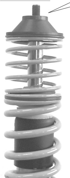
The original supporting bearing has to be put on the coilover strut and fixed with the supplied stop nut. Tightening torque for the piston rod is 35 Nm (26 ft-lb). The strut has to be installed according to the manufacturers recommended settings regarding tightening torque and fixing specifications.
