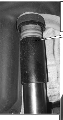
Mount the rear axle adjustment between spring and chassis, the original spring supporting disc is not longer used. You have to remove the rear axle adjustment to correct (screw up the threaded ring) the car height.
