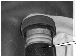
Tightening torque for the piston rod nut is 50 Nm (37 ft-lb). The damper unit has to be installed according to manufacturers recommended settings regarding tightening torque and fixing specifications.
