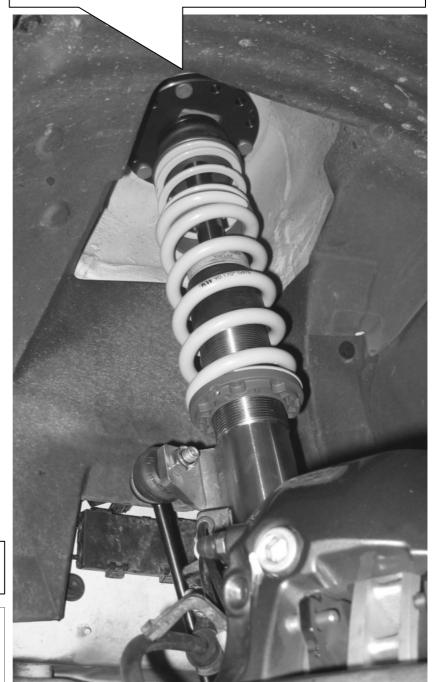
Tightening torque max. 22 Nm (17 ft-lb).
