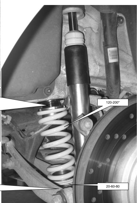
Use the supplied spring support at the bottom end of the spring.
