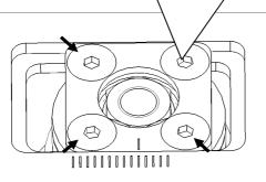
Distance collar: Please pay attention during installation of the distance collar that the clamping slot of the distance collar and the clamping slot of the wheel centre housing are laying one upon the other.
