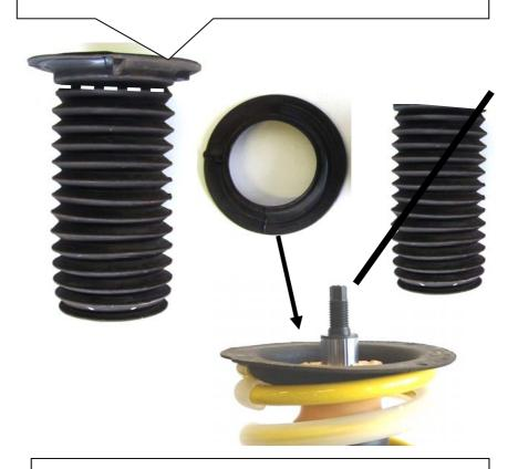
Put the standard supporting bearing unit with spring pad as shown in the picture and fix it with the supplied nut. Tightening torque for the piston rod is 40 Nm (29 ft-lb). Please install the strut unit to manufacturers recommended settings regarding tightening torque and fixing specifications.
