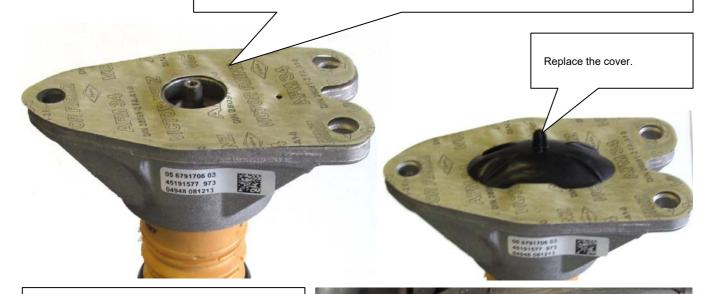
Mount the rear axle adjustment between spring and chassis, the original spring support is no longer used. You have to remove the rear axle adjustment to correct (screw up the threaded ring) the car height. Attention: Before the installation of the height adjustment perch the touching surface area have to be cleaned.
