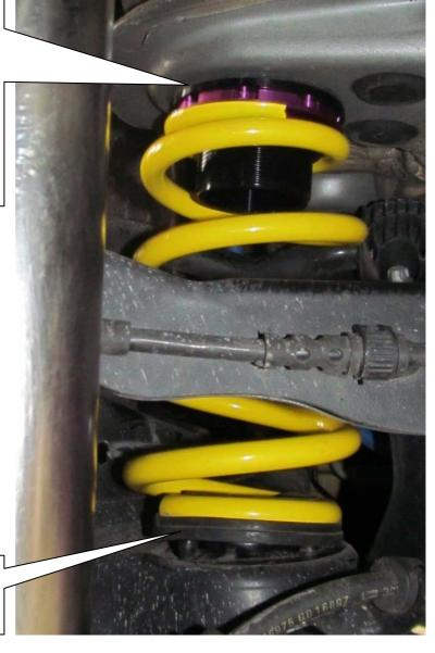
Use the original spring support at the bottom end of the spring.
