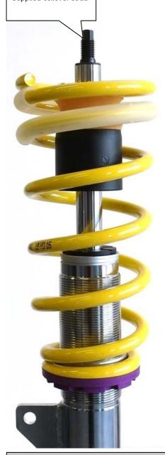
Cut off the standard dust cover on the dashed line. Insert the top part of the dust cover on the spring. The lower part of the dust cover is no longer required.
