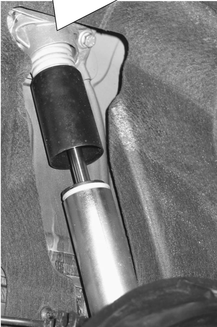
Mount the rear axle adjustment between spring and chassis, the original spring support is no longer used. You have to remove the rear axle adjustment to correct (screw up the threaded ring) the car height.
