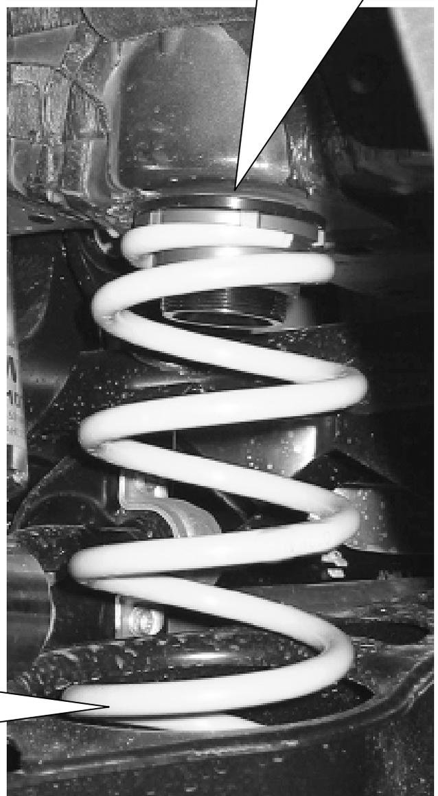
Use the original spring support at the bottom end of the spring.
