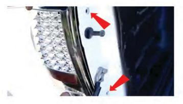
7) Reinstall the two phillips head screws that secure the tail lights.
