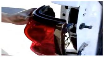
2) Unseat the tail light. Remove all three bulb sockets from the OEM tail light housing and set it aside.
