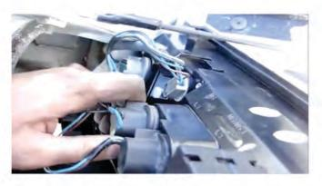
5) Reinstall the reverse lamp bulb and brake lamp bulb sockets into the SPYDER taillight housing. Be sure to twist the sockets securely into place.
