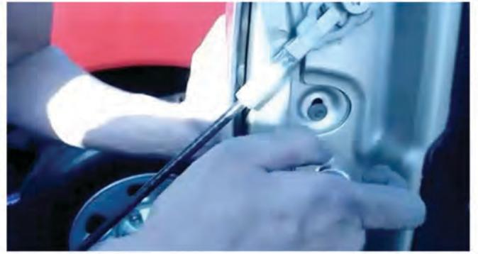
6) Reinstall the two T25 Torx Screws to secure the tail lights. Close the tailgate.
