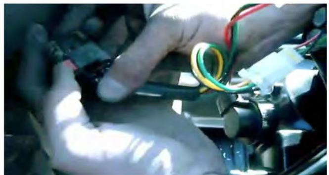
4) Locate your SPYDER tail light. Connect the SPYDER tail light harness to the OEM tail light harness. Slide the locking
