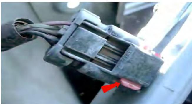
3) Disconnect the tail light harness by sliding the red locking tab free.
