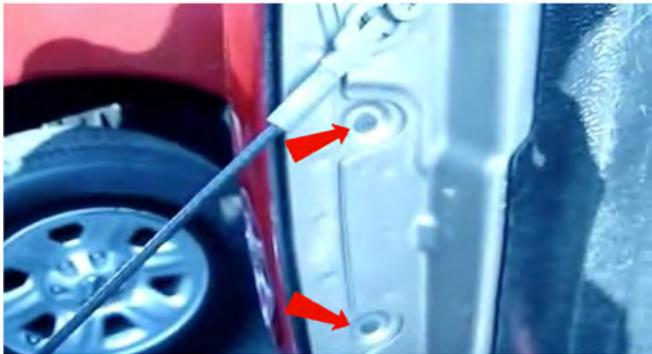
1) Open the tailgate. Remove the two T25 torx screws securing the OEM tail lights.
