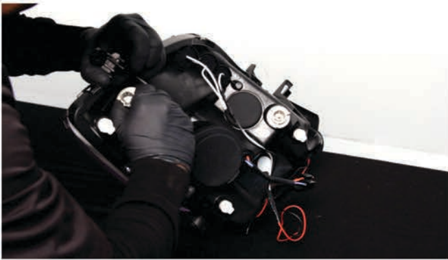
13) Install the turn signal socket into the Spyder headlight.
