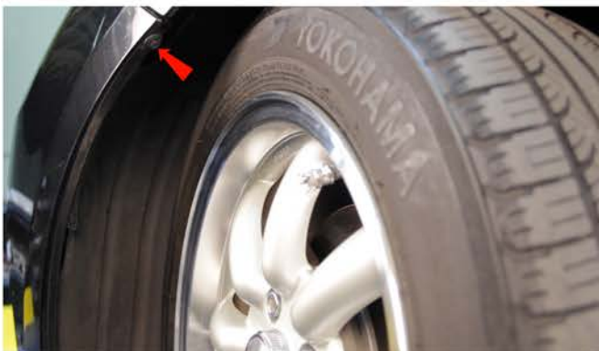
3) Remove [1x] phillips retainer securing the fascia at the wheel well.
