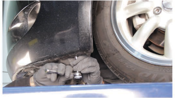
24) Reinstall [1x] 10mm bolt that secures the bottom corner of the fascia on each side.
