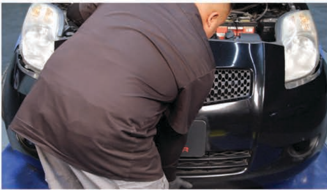
7) Unseat the bumper fascia by pulling the edges out then easing it back. If equipped with foglights, disconnect them. Then remove the fascia and set it aside.
