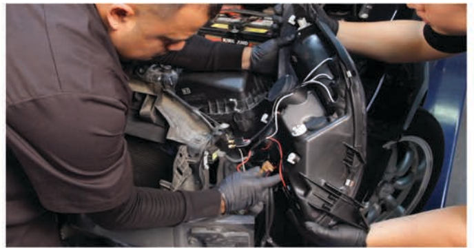
16) Reconnect the headlight harness, city light harness and the turn signal harness. The side-marker harness is no longer used.
