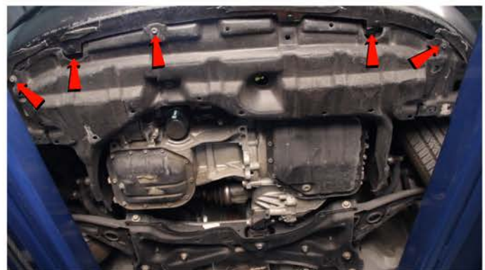
4) Remove [5x] 10mm bolts securing the fascia to the undertray.
