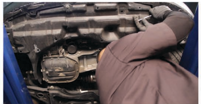
22) Reinstall [5x] 10mm bolts that secure the fascia to the undertray.
