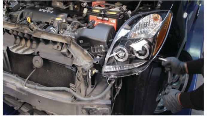
18) Reinstall [3x] 10mm bolts to mount the headlight.
