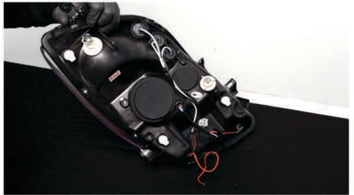
14) Install city light socket into the Spyder headlight.
