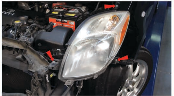
8) Remove [3x] 10mm bolts securing the headlight.
