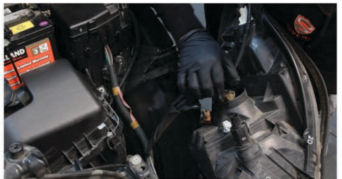
10) Disconnect the headlight, turn signal, side-marker and city light harnesses and remove the harness retainer.
