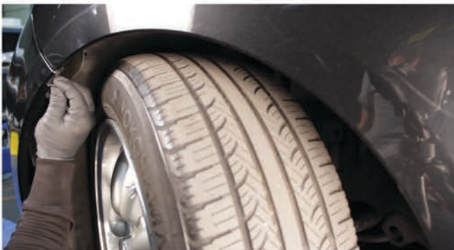
21) Reinstall [1x] phillips retainer securing the fascia in the wheel well.
