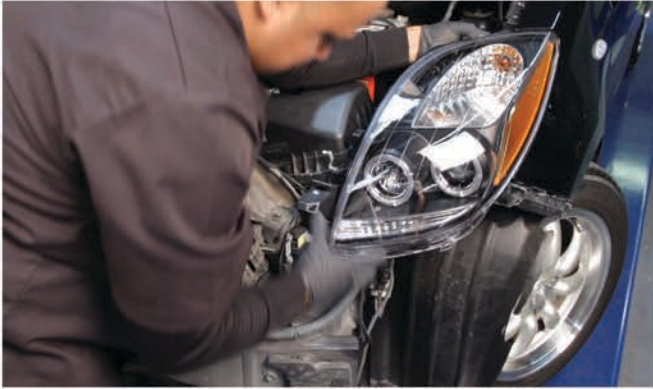
17) Seat the Spyder headlight, being sure the retainer tabs snap into place.
