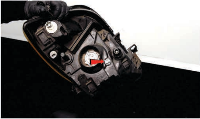
11) Remove the city light socket from the OEM headlight. Never touch exposed bulbs with bare hands.
