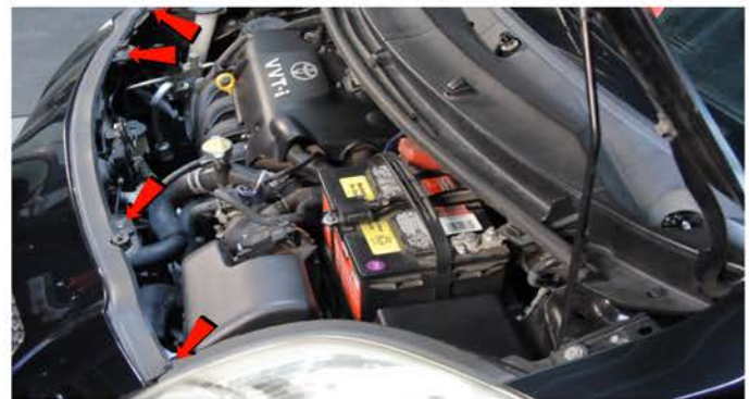
2) Remove [4x] Phillips retainers securing the fascia.
