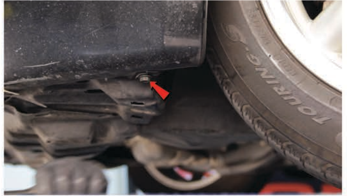
6) Remove [1x] 10mm Bolt securing the bottom corner of the fascia on each side.
